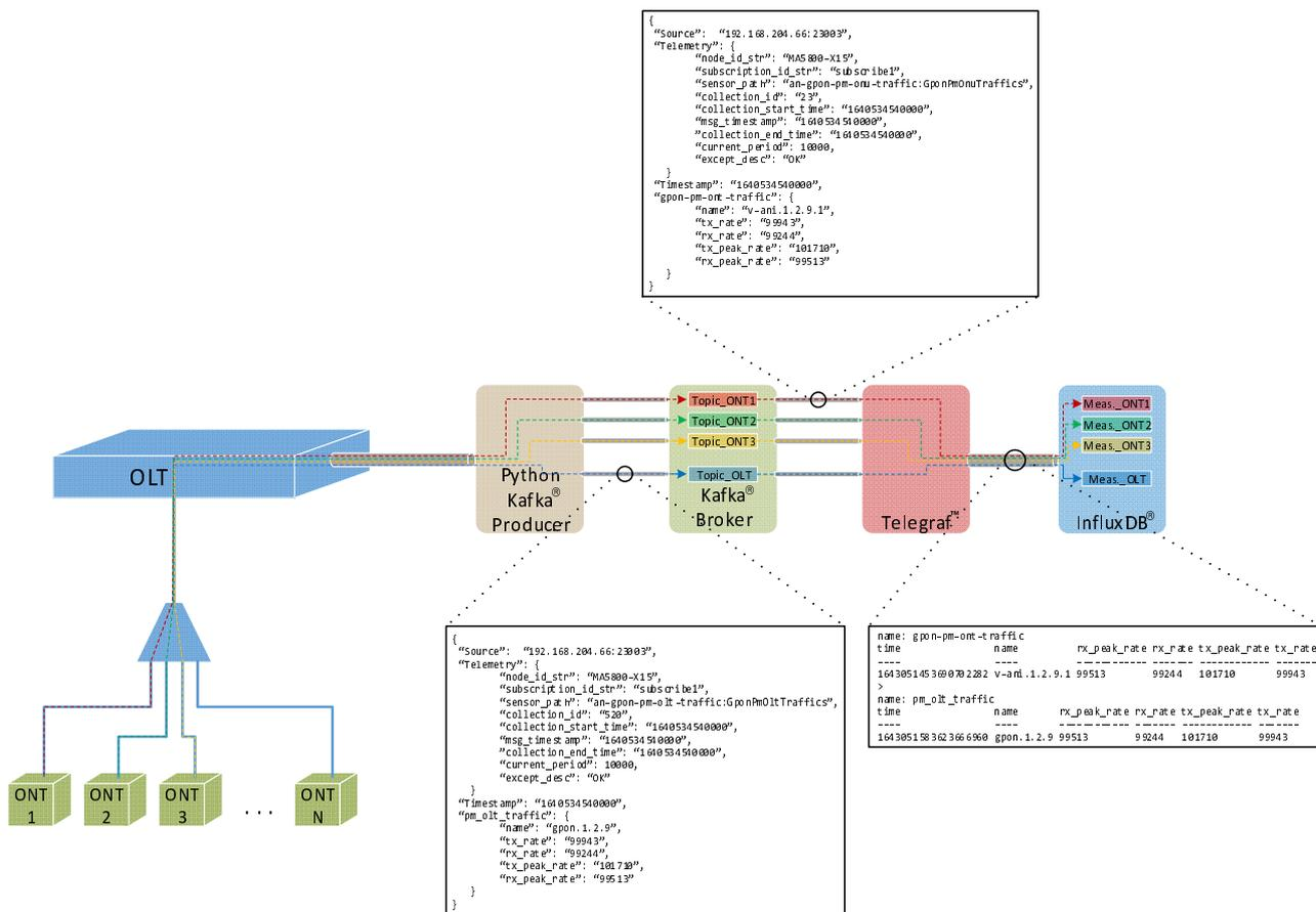
NOTE: The distribution of events into different topics based on their origin source/sensor path and further translation of events into measurements into the TSDB.
