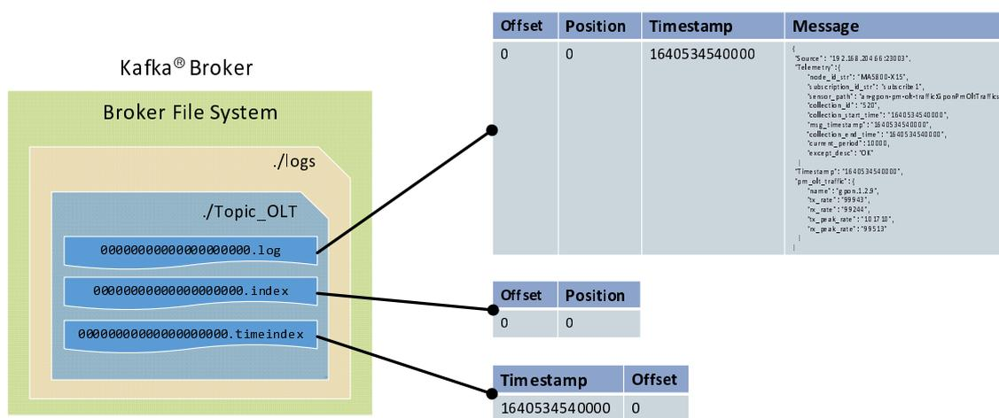
NOTE: The structure of a Kafka<sup>®</sup> topic with the corresponding log files.
