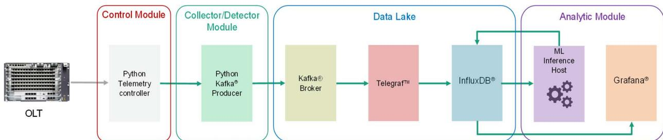
**Figure B.1: Functional blocks of the proposed telemetry streaming workflow and ML pipeline**
