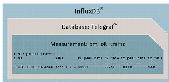
**Figure B.5: Structure of an InfluxDB<sup>®</sup> database with a corresponding measurement example**
