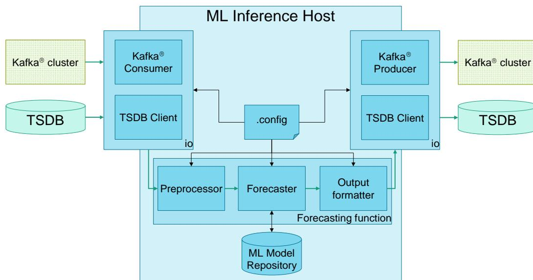
Figure B.7: Architecture of the ML inference host
