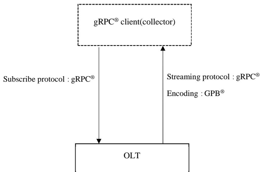
NOTE: Encoding methods other than GPB® are possible.
