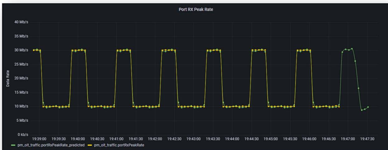
**Figure B.8: Evolution of a single telemetry parameter (i.e. port Rx Peak Rate) and its forecasted value over time**
