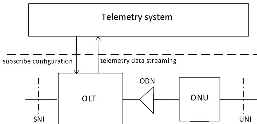
**Figure 2: Telemetry architecture in the Access Network**
