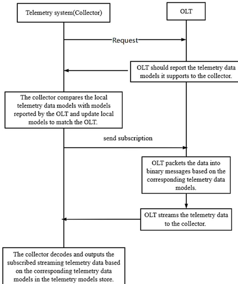
**Figure 7: Communication Process between OLT and Telemetry System**
