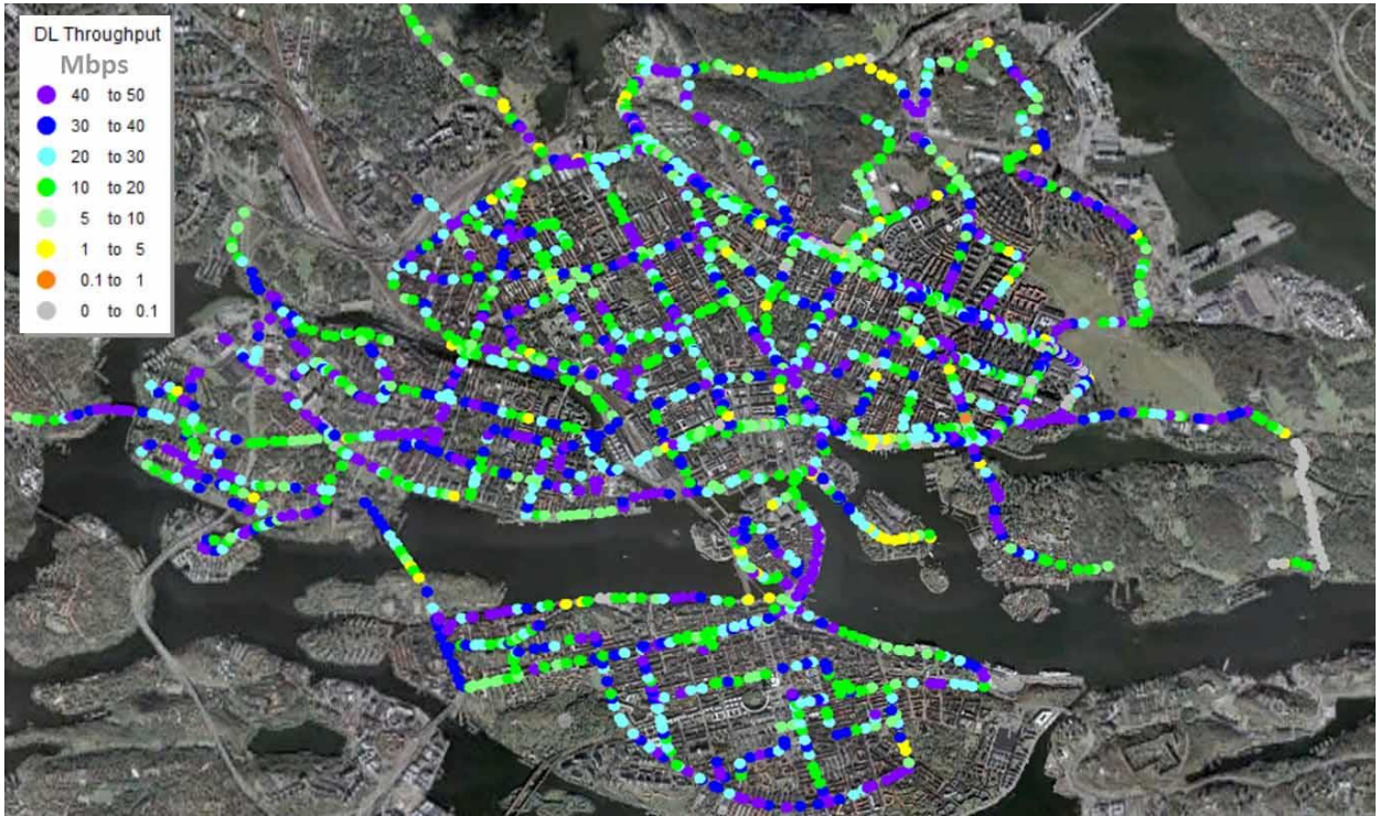
Figure 67: Drive Test of Commercial European LTE Network (10+10 MHz) 137
